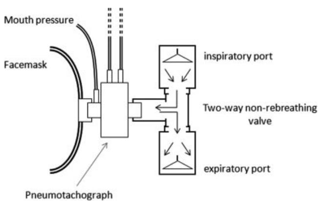
**Fig. 1. Diagrammatic representation of the equipment used to measure cPimax and cPemax. The inspiratory port on the two way non-rebreathing valve was occluded during the preceding expiration when measuring cPimax. The expiratory port was occluded during the preceding inspiration when measuring cPemax.**
