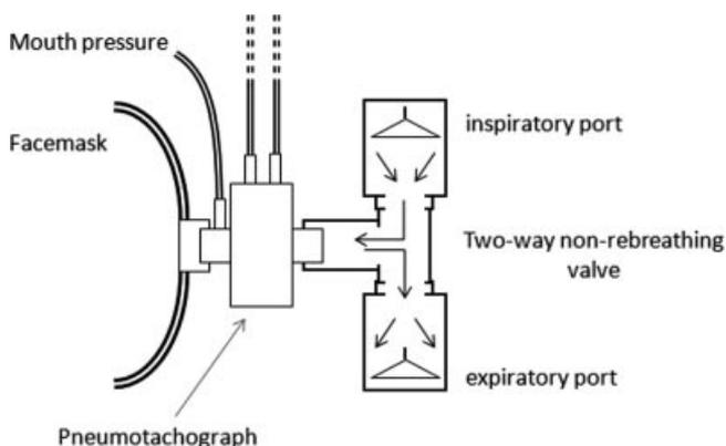
**Fig. 1.** Diagrammatic representation of the equipment used to measure cPimax and cPemax. The inspiratory port on the two way non-rebreathing valve was occluded during the preceding expiration when measuring cPimax. The expiratory port was occluded during the preceding inspiration when measuring cPemax.
